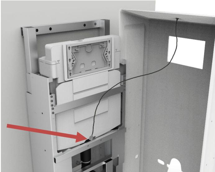
**b.** Guide the cable along the front of the lifting unit and pull it behind the cross bar below the cistern, as indicated on the illustration.
