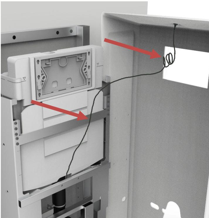
**d.** Use the attached strips to secure the wire to the belt as indicated. Roll up the remaining wire and strip it together in a bundle, as close to the top of the cover as possible.
