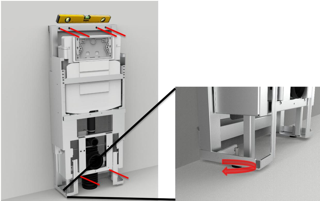
**a.** Line up frame with adjustment screws. Mark out 6 holes and drill holes for appropriate rawplugs. Ensure that the center of the bottom 2 holes is at least 130mm above the floor
