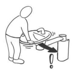
Ropox Swing Wash Basin has a turning function, which means that it is **NOT** allowed to be used as a walking or standing support.
