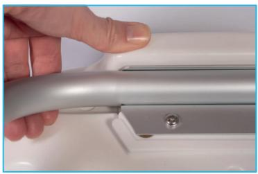
1. Use you thumb and fingers to gently lever the seat frame out of the seat frame stop.
