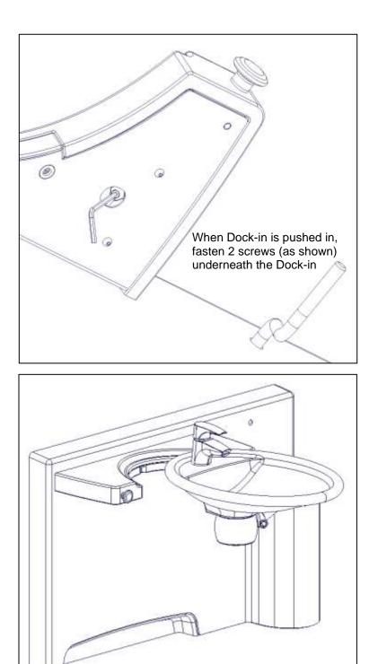
Test that washbasin freely can be swung into Dock-in and locks like it should. If washbasin is not positioned satisfactorily, fittings of Dock-in have to be loosened & either raised or lowered a little.
