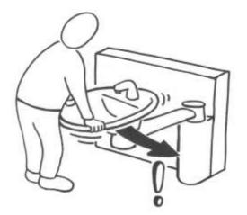
Ropox Swing Washbasin has a turning function, which means that it is  $\underline{NOT}$  allowed to be used as a walking or standing support.
